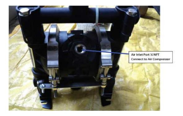
Diaphragm pump known as a Membrane pump, Air Operated Double Diaphragm Pump (AODD) or Pneumatic Diaphragm Pump. This is a positive displacement pump that uses a combination of the reciprocating action of a rubber, thermoplastic or teflon diaphragm and suitable valves. We supply all size of Diaphragm pump.
