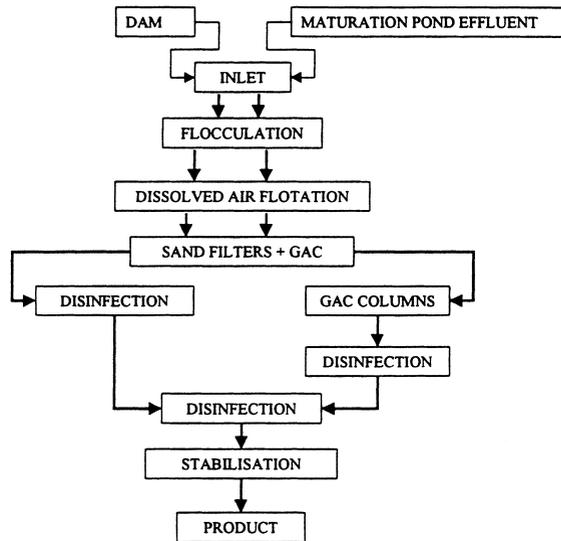
Figure 3 GRP flow diagram
