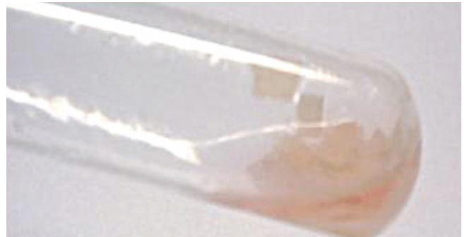
Membrane oxidation damage
